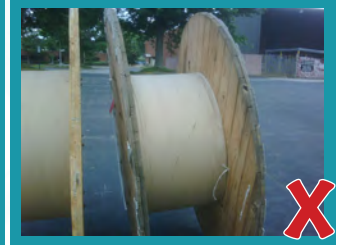
Loose Hub & lopsided
